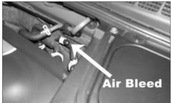
Figure 10. In the small open area between the plastic and the cowl is this air bleed for the heater circuit on the Infiniti FX. We've seen this type on other Japanese cars too; if you have an air pocket causing poor heater output, it's worth trying to find a bleed.
