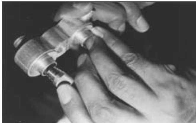
Figure 12. The AirSept kits use sizing gauges that enable the technician to pick the right screen for the compressor manifold's suction port. The early kits with three screens were for GM systems with Delphi compressors and the sizing gauge (shown) has just three steps. If this is used for other than Delphi compressors, you could select a wrong-size screen. The new kits, with eight screens, span a greater range and cover most systems, and contain a double-end design sizing gauge with a total of eight steps. However, most is not all, and even if the screen is supposed to fit an application, an occasional out-of-tolerance manifold port might not hold a screen. But the gauge tells you.
