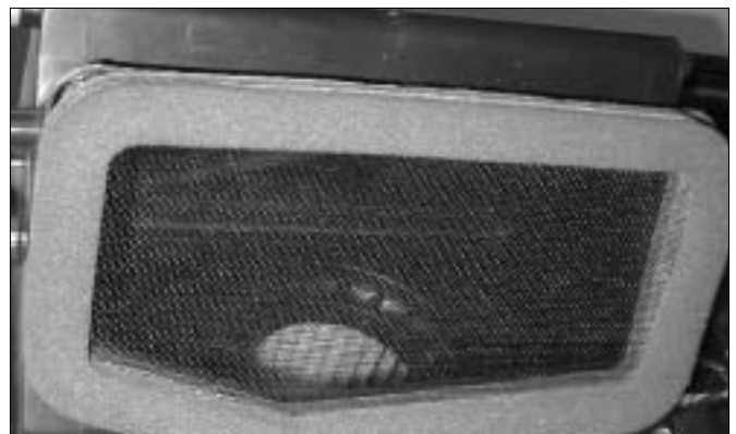
Figure 3. This air intake screen on a Saturn VUE gives you an idea of what GM is planning to release as a service part, and possibly as original equipment on vehicles without an air intake filter.
