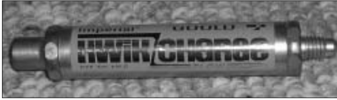
Figure 4. This is the old “Kwik-Charge,” which was sold to prevent compressor slugging from liquid charging into the suction side. We bought it in the days of CFC-12. It apparently has some sort of restriction to meter droplets of liquid refrigerant, and (what sounds like when we shake it) an anti-blowback valve in case it was connected to the high side.
