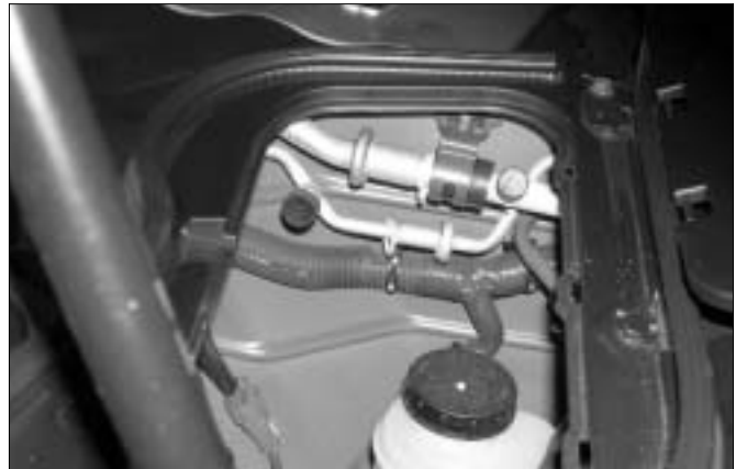
Figure 9. The cover is off and there's the brake fluid reservoir, all right. But both A/C service valves are there too.
