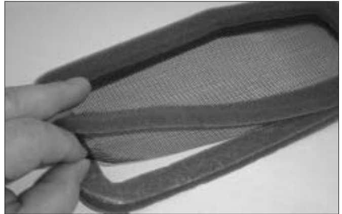
Figure 2. An air intake screen can be made from fine-mesh household screen sandwiched between layers of two-sided adhesive foam gasket material.
