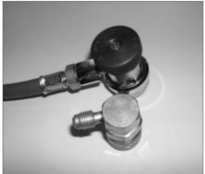
Figure 6. Two service hose couplings. The knurled knob on the larger one permits you to first install the coupling on the service valve, then turn the knob to push open the valve. The smaller one, although it goes into tighter quarters, may be more difficult to install because it requires a single push-on operation.
