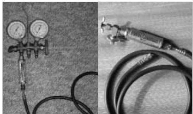
Figure 5. The “Kwik-Charge” inlet side was supposed to be threaded into the low-pressure gauge's male fitting on the gauge manifold (at left), with the service hose threaded onto the device's outlet and to the suction side service valve. More often, it was in line with the end of a small can tapper and service hose, as shown at right.
