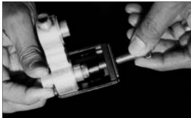
Figure 13. If you can push the screen in easily with your thumb, it's probably the wrong size. The screen should require press-in installation with this special tool.
