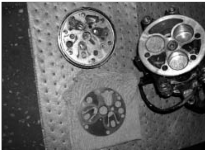
Figure 11. This compressor failed to perform for obvious reasons: broken suction reed valves. Could chunks of suction reed have blown back into the low-side hose? It didn't seem to have a restriction, but with this evidence from the compressor, why take a chance? Yes, the technician installed a suction screen to protect the new compressor.
