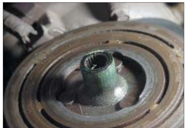
This clutch was removed from the Ford F-150 truck compressor. Sealer buildup on the clutch hub was substantial.
