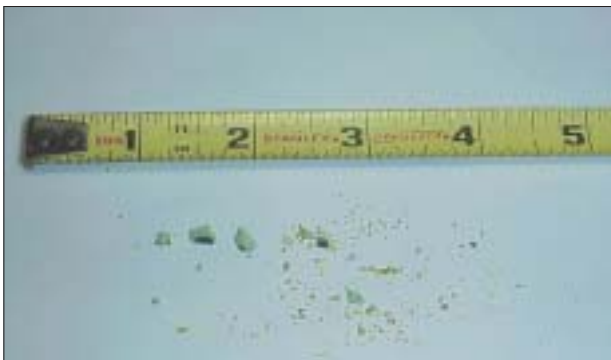
The particles below the tape measure were scraped from solenoid valves in a recovery/recycling machine. Lab tests showed the particles were a match for an A/C sealer.
