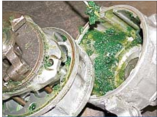
This compressor was disassembled and found to be full of green gel after return for warranty adjustment.
